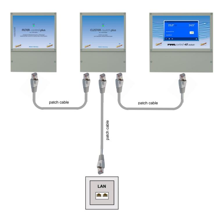
After connecting the cables and switching on the controls, a logical connection must be established between the devices. The details can be found in the installation and operating instructions for the corresponding devices. The two **resi** devices then exchange data via a local network.
